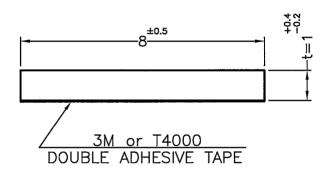
NOTE: 1. HEIGHT INCLUDE ADHESIVE TAPE, NOT INCLUDE RELEASE PAPER. 高度含肯膠但不含離型紙厚度.
