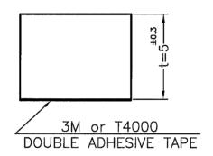
NOTE:1. Height include adhesive tape, not include release paper.
