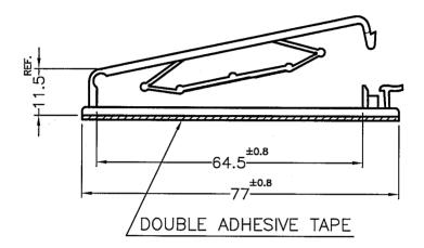
NOTE:1. THE PRODUCT SIZE IS NOT INCLUDED THE SIZES OF ADHESIVE TAPE AND ITS LINER. 產品尺寸皆不含背膠及離型紙.
