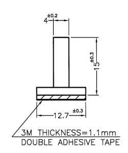
NOTE: 1. THE PRODUCT SIZE IS NOT INCLUDED THE SIZES OF ADHESIVE TAPE AND ITS LINER. 產品尺寸皆不含背膠及離型紙.
