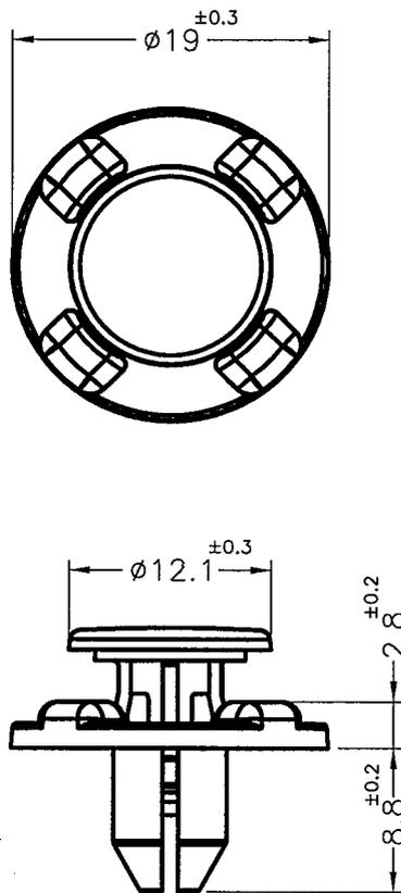
MOUNTING HOLE:  $\phi 7$ mm
