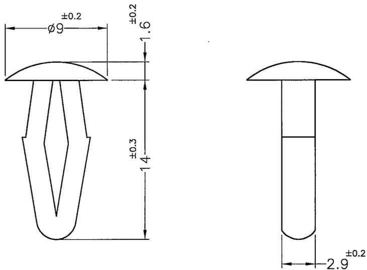
MOUNTING HOLE:  $\phi 3.9\text{mm}$
