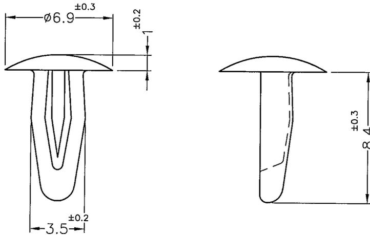
HOLE IN CHASSIS:  $\phi 3.1 \sim 3.2$ mm
