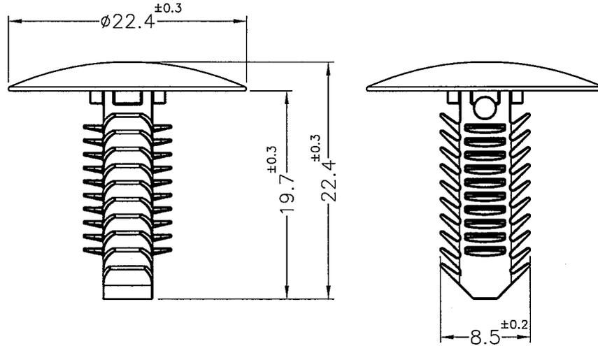
MOUNTING HOLE:  $\phi 7.9\text{mm}$
