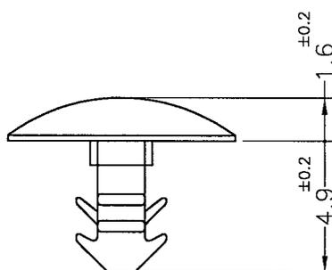
MOUNTING HOLE:  $\phi 3.0$  mm
