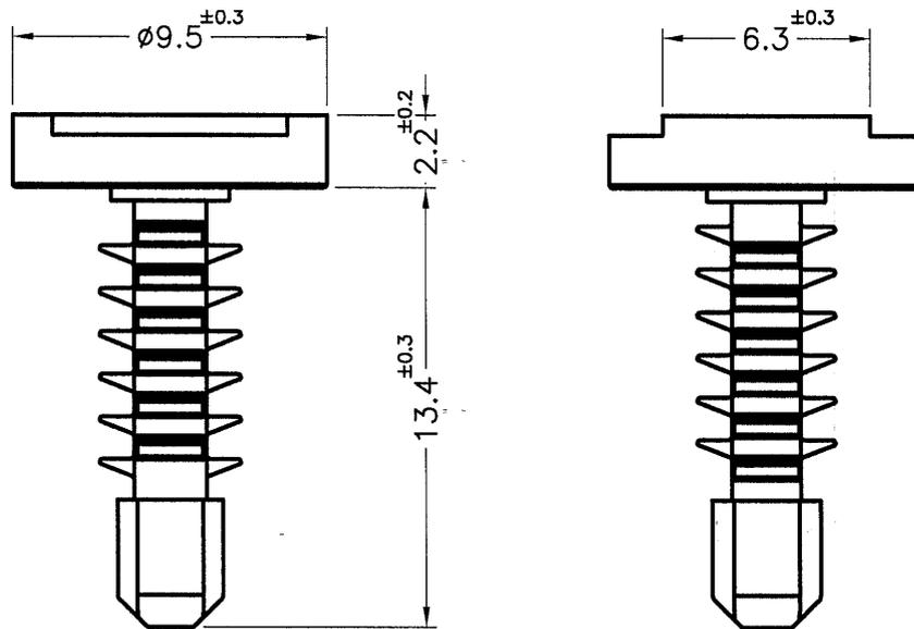
MOUNTING HOLE:  $\phi 3.96\text{mm}$
