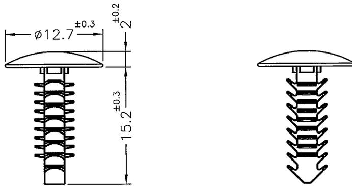
MOUNTING HOLE:  $\phi 4.8\text{mm}$
