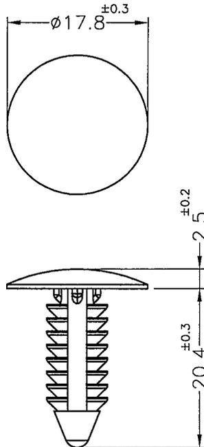
MOUNTING HOLE:  $\phi 6 \sim 6.3 \text{mm}$
