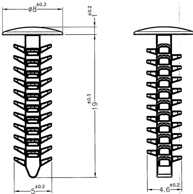
MOUNTING HOLE:  $\phi 4.0\text{mm}$
