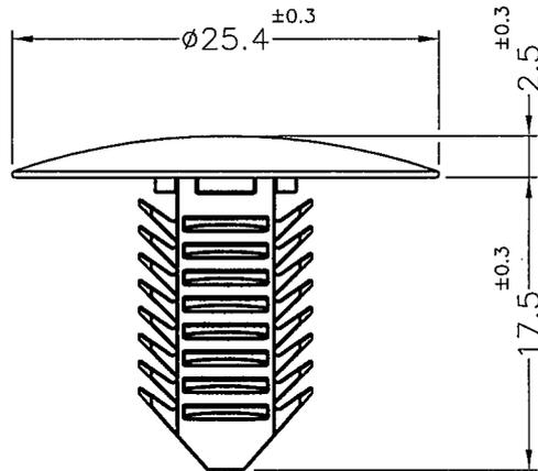
MOUNTING HOLE:  $\phi 9.5\text{mm}$
