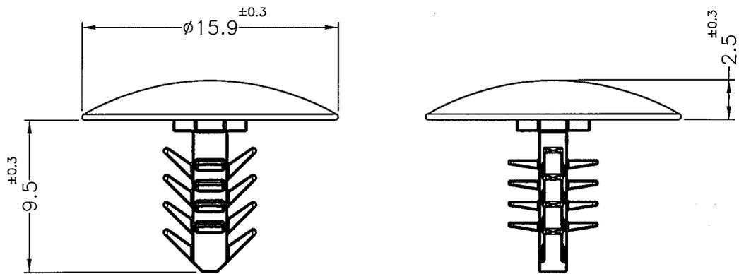
MOUNTING HOLE:  $\phi 5.25$  mm
