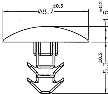
MOUNTING HOLE:  $\phi 3.2\text{mm}$
