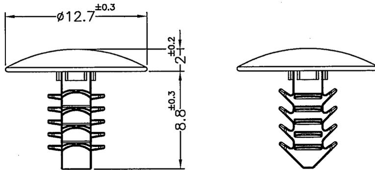
MOUNTING HOLE:  $\phi 4.8\text{mm}$
