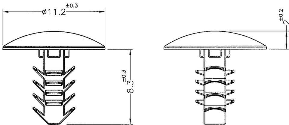
MOUNTING HOLE:  $\phi 4\text{mm}$
