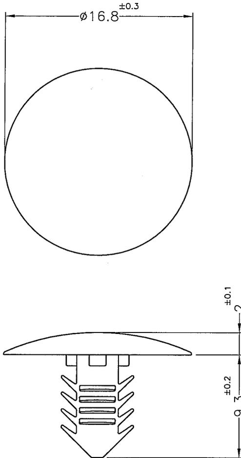
MOUNTING HOLE:  $\phi 6\text{mm}$
