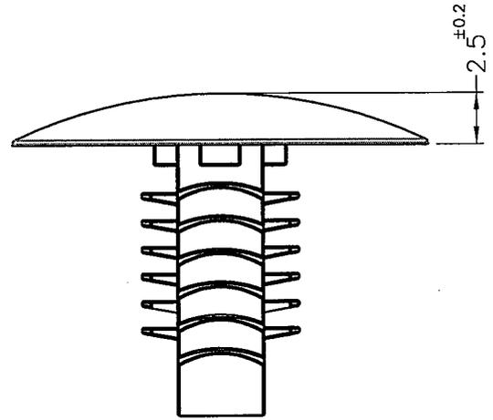
MOUNTING HOLE:  $\phi 7.1\text{mm}$
