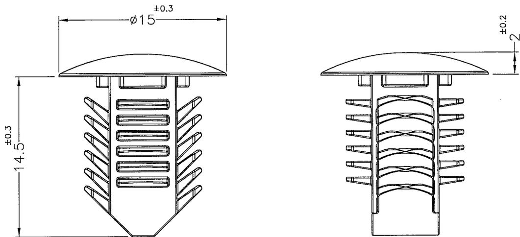
MOUNTING HOLE:  $\phi 10.0$  mm
