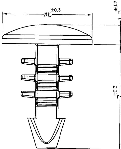
MOUNTING HOLE:  $\phi 2.7 \sim \phi 3.3 \text{mm}$
