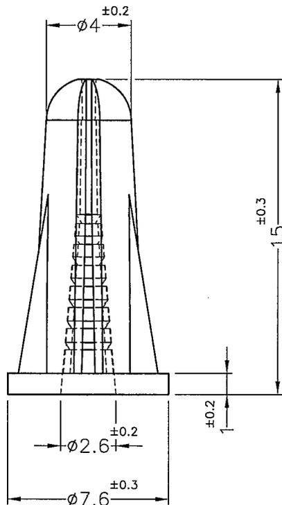
MOUNTING HOLE:  $\phi 4.8\text{mm}$
