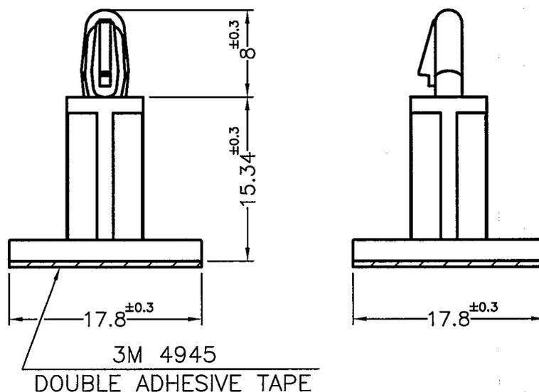
NOTE:1. IT IS HAND-CUT ADHESIVE TAPE, SO CAN NOT PERFECTLY STICK EVENLY. IT IS POSSIBLE TO HAVE SOME PORTION EXPOSED OR SHRINKING INWARD. THIS IS A NORMAL PHENOMENON.
