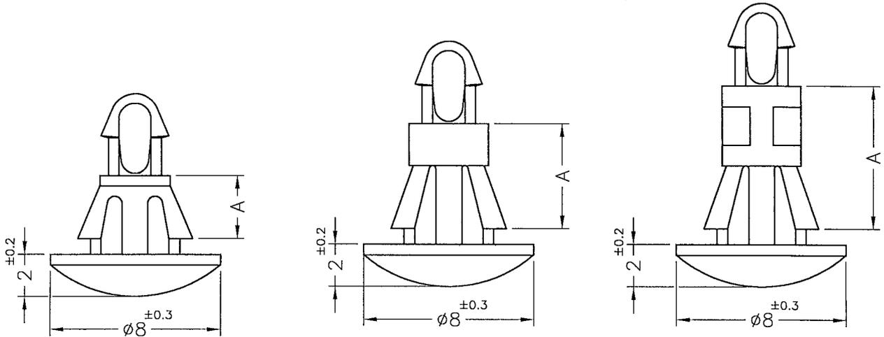
MOUNTING HOLE:  $\phi 4.0\text{mm}$
